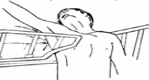
Zone 5 - Entrapment between split rails
