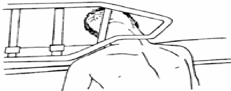
Zone 4 - Entrapment between top of compressed mattress and bottom of rail at end of rail
